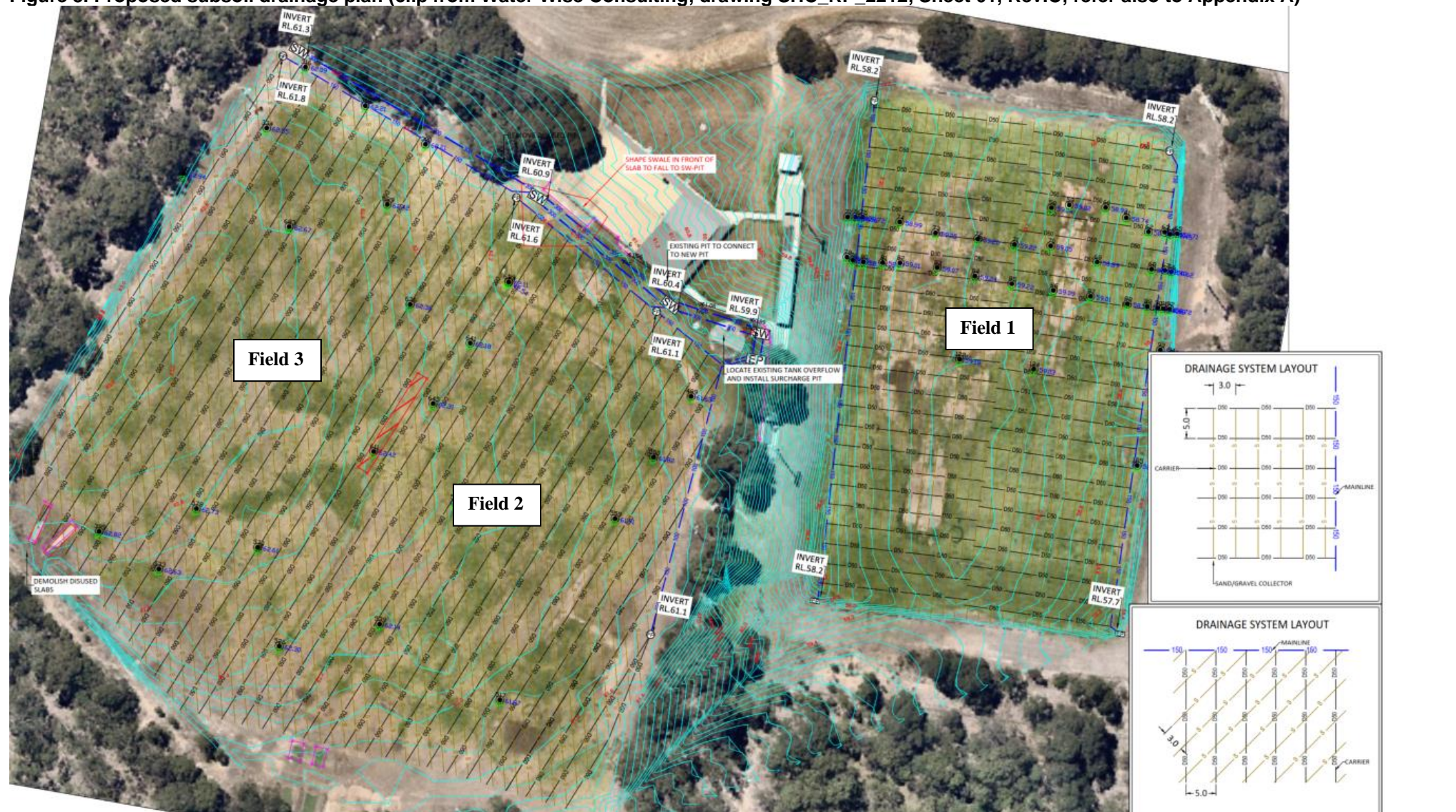
Figure 3. Proposed subsoil drainage plan (clip from Water Wise Consulting, drawing SHC_RP_2212, Sheet 01, Rev.C; refer also to Appendix A)
